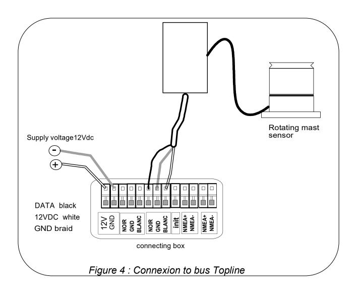
If you have to cut the bus cable, we recommend that the wires are tined connecting.
